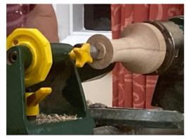
Dave then reversed the piece in the chuck and drilled a 6mm hole through the centre all the way through so that the wire for the lights could be threaded through.
